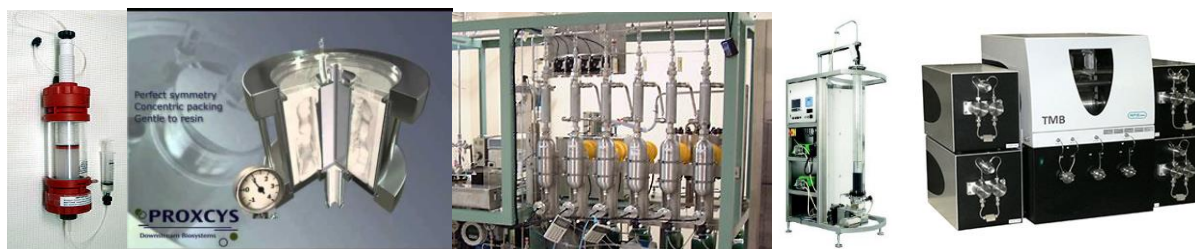
Figuur 11: A) Axiale kolom; B) Radiale kolom; C) SMB; D) EBA; E) TMB
